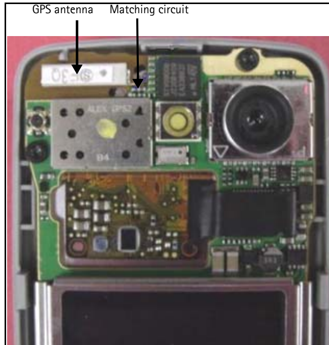
Figure 10: Position of the GPS antenna on the PWB
