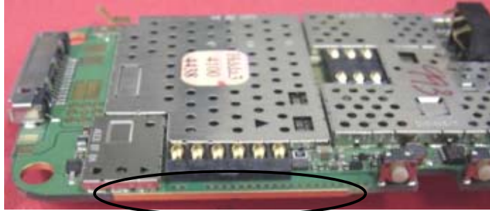
Figure 12: BT antenna on the PWB
