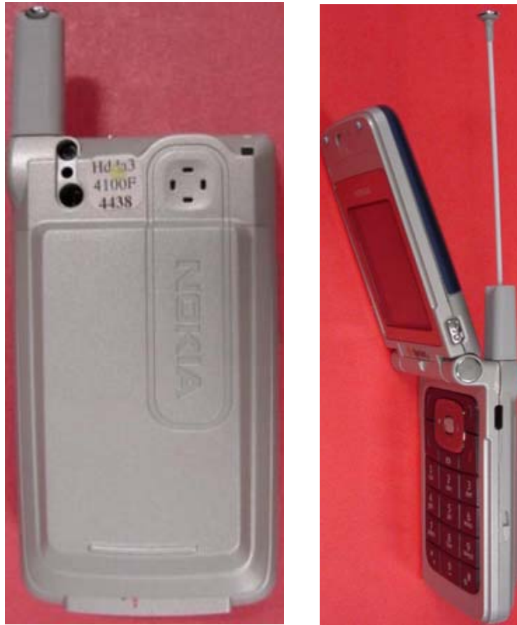
Figure 3: Whip retracted and whip extended
